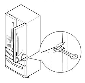
Level the refrigerator by using an 11/16 inch (18mm) wrench or a flat blade screw driver.
